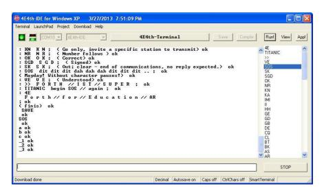
For completion we click on "OK" at the Wordlist (right panel), then a click on "App!", and from now on we will be greeted with an "OK" Morsecode each time when we hit the LaunchPad RESET button or when we connect our LaunchPad to power again:
