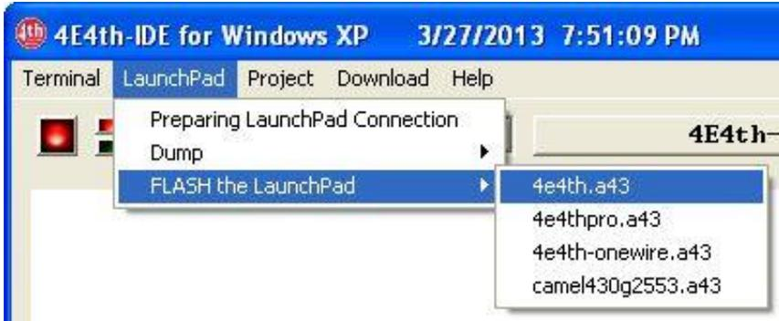
This menu point is used to "FLASH the LaunchPad" and allows to put 4E4th Forth program onto the LaunchPad, using one of these files, which are residing in the folder \Engine\Flasher.
