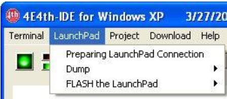
LaunchPad has three submenus: "Preparing LaunchPad Connection", "Dump", and "FLASH the LaunchPad".
