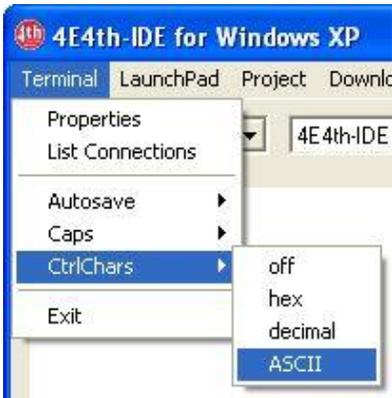
The "CtrlChars" setting allows to see control characters sent to and from the target.
