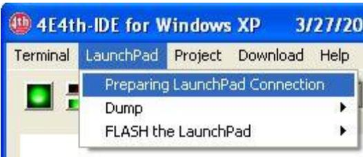
Preparing LaunchPad Connection is needed, when a LaunchPad is connected to a PC for the first time,
