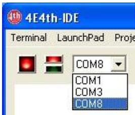
When starting 4E4th-IDE.exe, the connection check is automatically done.
